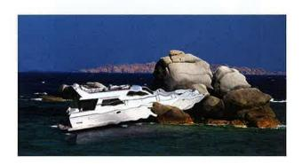
There are different degrees of being aground. You can be "hard grounding" meaning you hit so hard that part of the hull embedded into the sea bottom, the hull may be breached (has a hole). "Soft grounding" means you bumped the bottom, or moved into a very soft type of bottom, such as sand or mud. Actions to take if aground:
